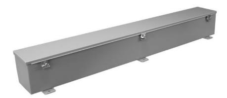
**Construction:** C & I Enclosures Type 12 Hinge Cover Wiring Trough is fabricated in accordance with UL specifications from code gauge steel. An oil resistant gasket is attached to the cover to prevent dust from entering the trough. The cover is attached to the body with butt hinges on one side and external screw clamps on the other. All seams are continuously welded and ground smooth.
