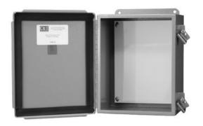
Construction: C & I Enclosures Type 12 Painted J.I.C. Continuous Hinge Boxes are fabricated in accordance with U.L. specifications, from code gauge material. An oil resistant gasket is attached to the cover to prevent dust from entering the box. The boxes are provided with a continuous hinge and external screw clamps on one side. All seams are continuously welded and ground smooth. External mounting feet are provided along with studs for mounting optional panels.
