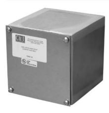
Construction: C & I Enclosures Type 12 Screw Cover Gasketed Boxes are fabricated in accordance with U.L. specifications from code gauge material. All seams are continuously welded and ground smooth. An oil resistant gasket is attached to the cover to prevent moisture or dust from entering the box.
