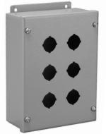
**Construction:** C & I Enclosures Type 12 Pushbutton Enclosures are fabricated in accordance with UL specifications from code gauge steel. An oil resistant gasket is attached to the cover to prevent dust intrusion. All seams are continuously welded and ground smooth.
