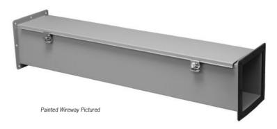
Construction: C & I Enclosures Type 4X Stainless Steel Feed-Through Wireway is fabricated in accordance with U.L. specifications from code gauge material. An oil resistant gasket is attached to the cover to prevent dust from entering the wireway. The cover is attached to the body with butt hinges on one side and external screw clamps on the other. All seams are continuously welded and ground smooth.
